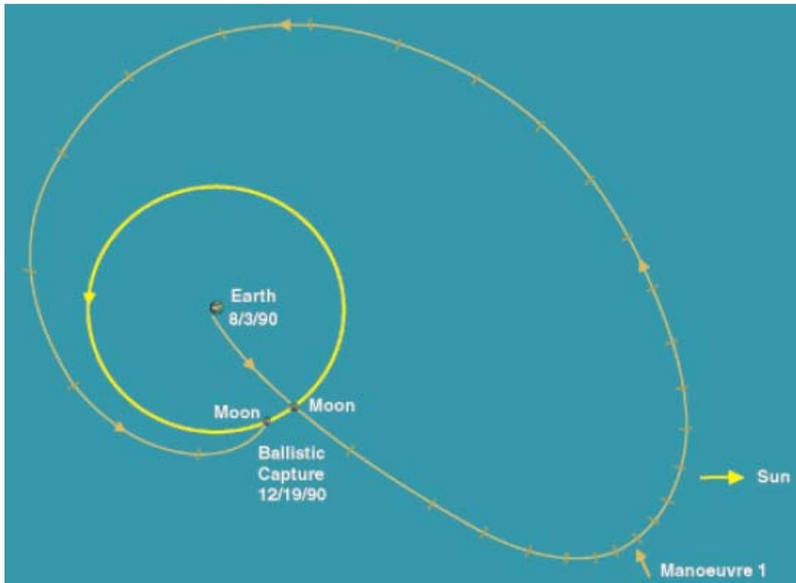
Figure 7 Hiten transfer trajectory [3]
