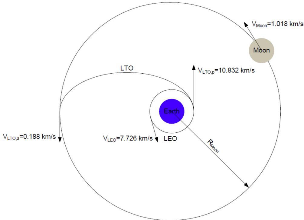
Figure 4 Hohmann transfer to Moon (Velocities for 300 km LEO and 384400 km circular Moon orbit)
