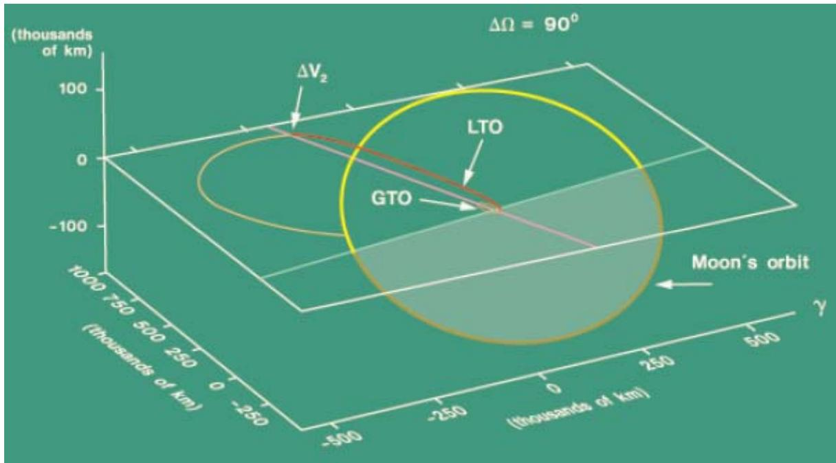
Figure 6 Bi-elliptic transfer from GTO [3]
