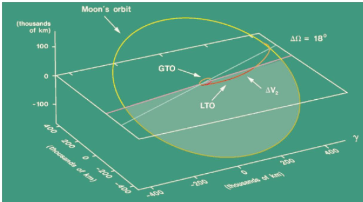
Figure 5 Direct transfer from GTO including mid-course manoeuvre [3]
