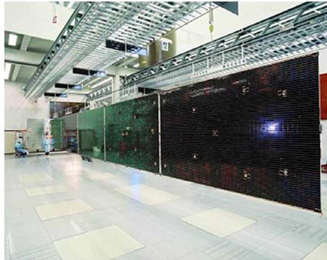
Figure 20 Eurostar 3000 solar array [10]
