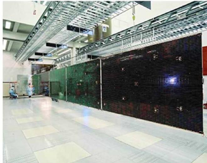
Figure 20 Eurostar 3000 solar array [10]
